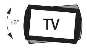
A screwdriver to adjust the screw, control the tilt angle of the TV, the angle can be controlled at ±3°.
