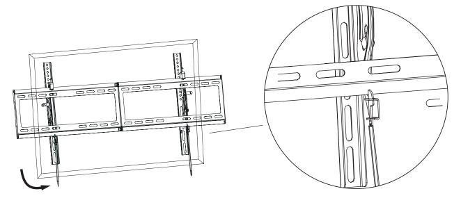
Note: after the upper hook is hooked, push the TV back until the safety lock is tightened, as shown in the picture.
