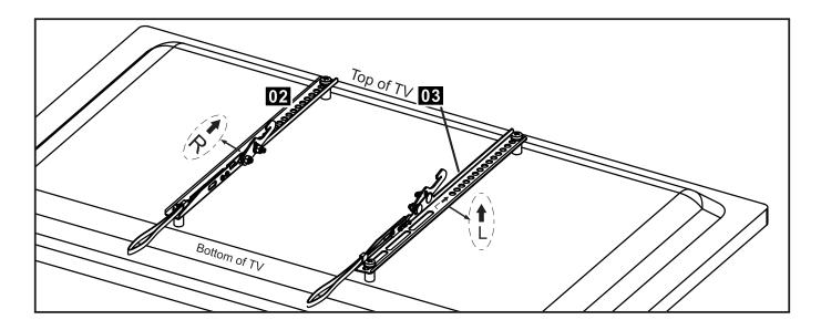
Please adjust the tilting angle with the Allen wrench for both (2) and (3) as the pictures show before hanging monitor.
