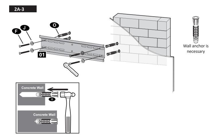
Install wall plate (1) using lag bolts (F) and washer (J) and anchor (O). Tighten the lag bolts (F) until they are pulled firmly against the wall palte (1).
