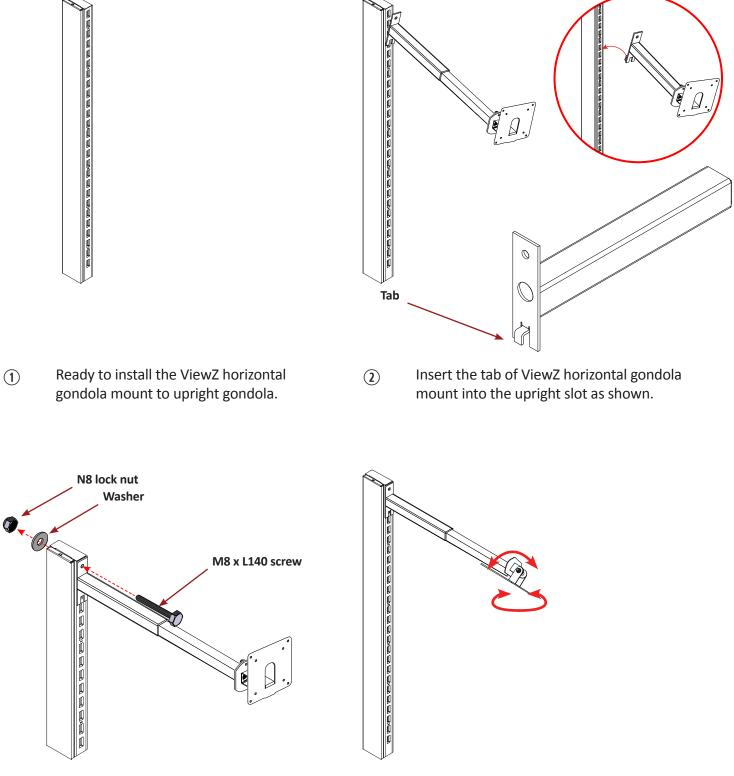
Lock the ViewZ horizontal gondola mount to gondola upright by using bolt & nut.
