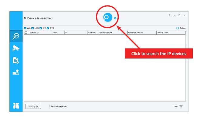
It will search for IP devices on the same network, and show the "Device ID", "IP Address", "Product Model" and "Software Version"
